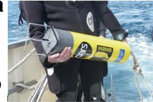
Hydrophone : underwater passive acoustic sensor
